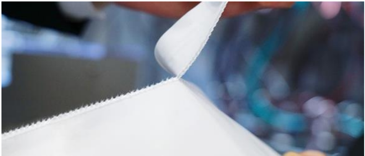
Figure: The HDG pressure seal module can process the uncoated paper "NexPlus MC" with no sealing layer into bags. / Source: HDG-Verpackungsmaschinen
