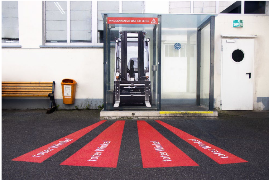
Caption: The field of vision of forklift operators is extremely limited, which the red bars on the ground clearly show. Image rights: Koehler Group
